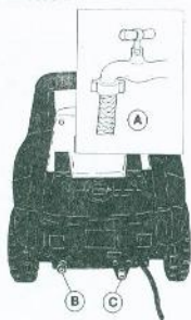
Water circuit connection.
