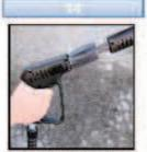
Release any pressure in hose by squeezing trigger and disconnect hoses from machine.
