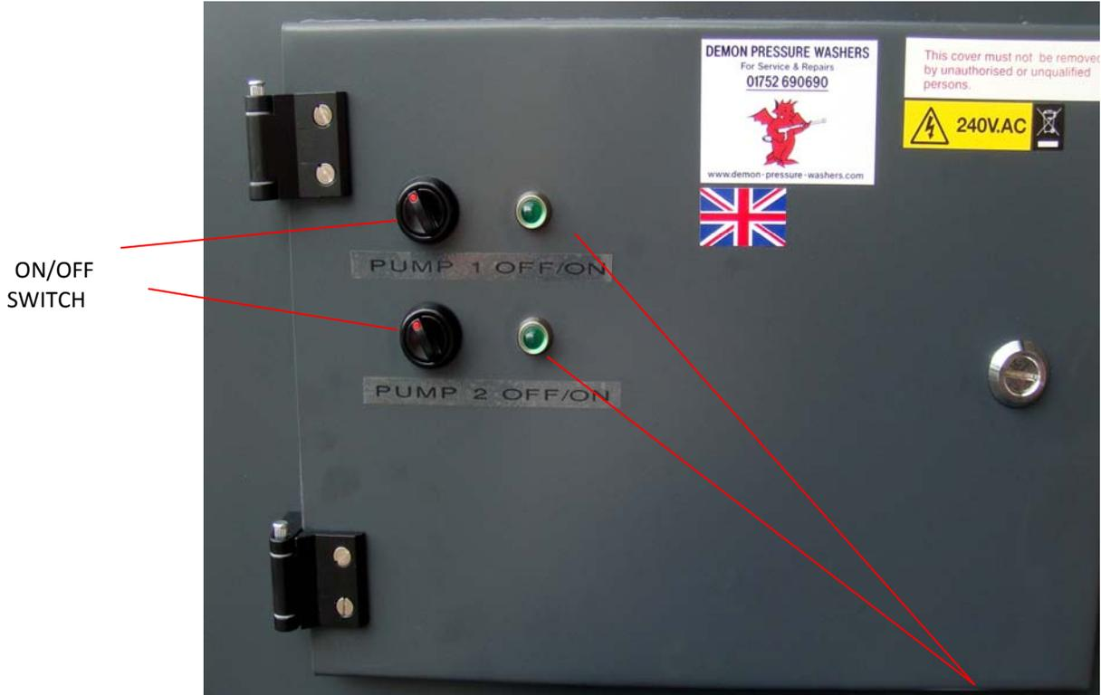
N.B. If there is no water in the machine a light will still indicate power but will not be operational. CHECK WATER
